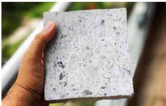
laboratory are mixed with the shredded PPE waste. "The mixture is set aside for about six hours before setting it in moulds. The moulds are dried for a few days before use," elaborates Desai, who claims that Brick 2.0 is fire retardant, recyclable and absorbs less than 10 per cent water.
